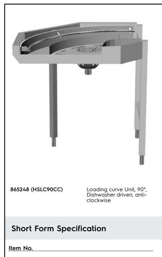
Constructed in 304 AISI stainless steel. Basin with sloping bottom and drain. Feeding bar. It is driven by the dishwasher. Square 40x40mm tubular leg on heightadjustable feet. Designed for 500x500mm dishwashing baskets. Knock-down delivery. Basket feed direction: anticlockwise.
